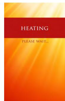
When machine temperature reaches brew temp, display will change to the Drink Instruction Screen. The machine is now ready for operation.
