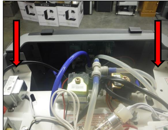
9. Disconnect tubing from inlet elbows on both solenoids and allow water to drain.
