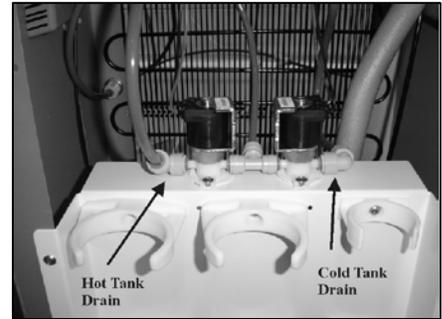
9. Reconnect tubing into inlet elbows once drained.
