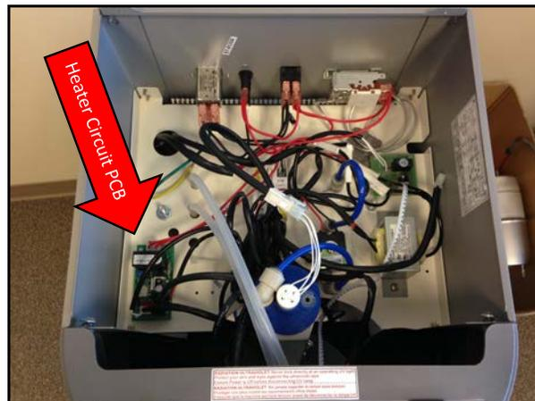
2. **WL350** comes with Sleep Mode active with Jumper JP7 in the "ON" position (Pin 1 and 2) on the Heater Circuit internal Printed Circuit Board (PCB). Deactivate the sleep mode function by moving PCB Jumper Pin JP7 – Part Number 20-1005 to the "OFF" position (Pins 2 and 3).
