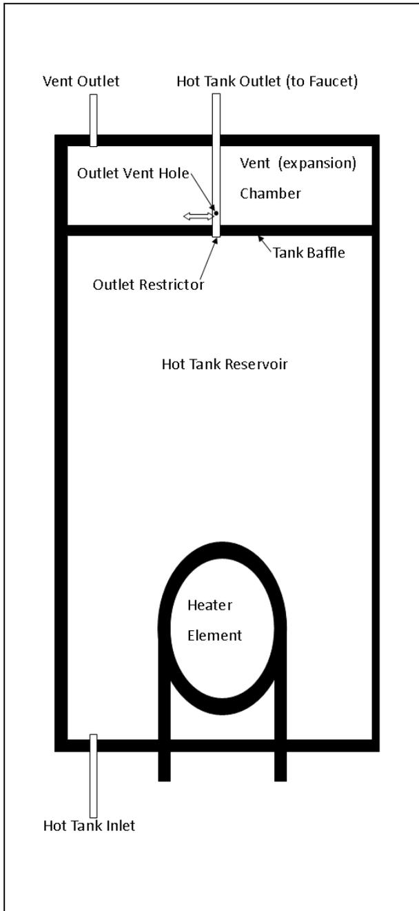
All **Waterlogic** Hot Tanks have a built in Vent or Expansion Chamber in the top of the tank except for WL270 (GF) units.
